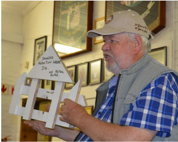
Douglas Lock produced a routing jig for cutting repetitive grooves. Douglas endorsed the use of a pinner for easy and quick construction of such jigs.
