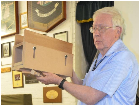
Paul Roberts made this unit which fits on a lathe and is used in conjunction with a router to make accurate dowels.
